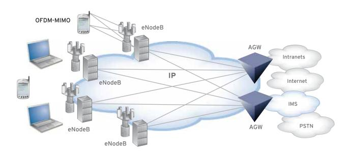
A typical LTE/SAE network will have two types of network elements supporting the user and control planes.
